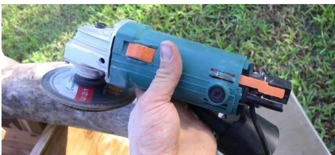
An unsafe angle grinder – note the missing guard, the "always-on" switch and exposed electrics.
