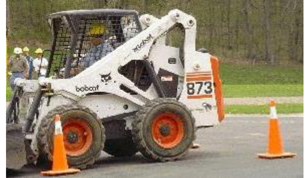
Cones or barriers should be used to establish an exclusion zone around mobile plant and equipment.
